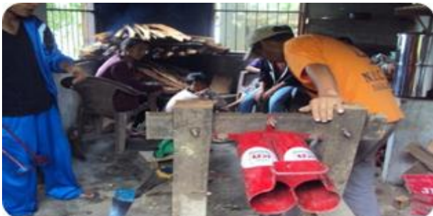
Figure 6. Fabrication of frame of Treadle pump and its input to Jalkund.
